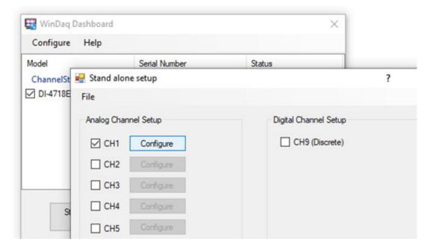
In the Configure window, enter 247 and 0 for Sensor Output, and 0.5 and 0 for Sensor Input (as shown below). Change engineering units to 'L/sec'.
