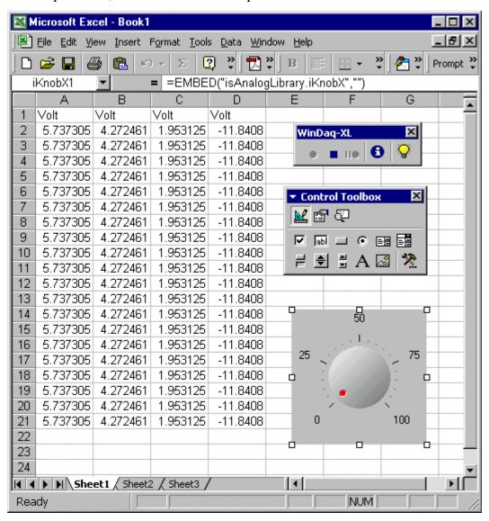
3. When the control is placed, you are automatically in "Design Mode". Right click on the control and select "Properties" or just press the Properties button in the Control Toolbox. Here, you can change many properties of your control, such as size, style, font, etc., but, most importantly, you can link the control to your application. Next to "LinkedCell", type in the
