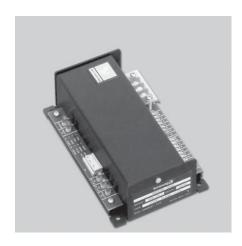
This unit isolates and boosts RS-485 signals to extend communication distances or increase the number of devices on the network. Each Repeater permits the addition of a network branch with up to 32 devices (including the Network Repeater) and will transmit RS-485 signals another 4000 feet. Operation is transparent to all devices and no handshaking is required. Two terminal blocks are provided for 120 ohm resistors to terminate both ends of the network branch.
